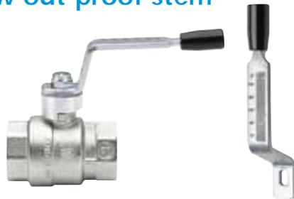
The **BASIC•HT** ball valves are bottom loaded stem designed. This "anti-blow-out" stem offers more guarantees against the accidental release of the stem and it prevents from tampering with the internals of the valve.
